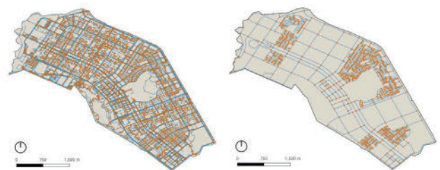
Figure 6. Comparison of measurement of street connectivity by data (Ilsan New Town, Left: OSM, Right: SAD) OSM: Open Street Map, SAD: Street Address Data
