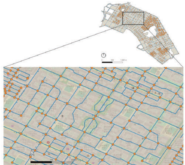
Figure 8. Measurement of street connectivity – 4th Approach including the streets within the residential area (Ilsan New Town)
