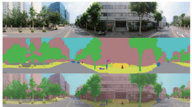
Figure 7. Example of elements extracted by semantic segmentation
